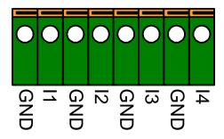
To insert or remove a wire, use a small flat-head screwdriver and press in against the orange lever. While holding the lever, insert or remove a wire into the desired terminal. Release the orange lever when finished. If you inserted a wire, give the wire a tug to be certain it is properly clamped in the terminal.
