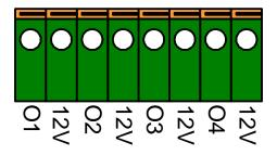
Current from the 12V supply is limited to 500ma by an internal PTC fuse. The 12V supply terminals may be used for powering external devices (PIR motion sensors, etc.). The total current draw of all attached devices from the 12V supply must be less than 500ma.
