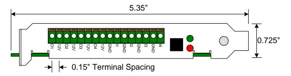
Drawing of board from top side showing connectors:
