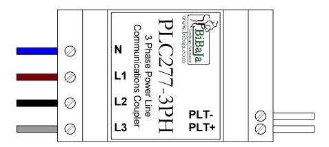
Connect low voltage power line coupling circuit (30VAC/42VDC maximum) to PLT-/PLT+ terminals (Connections shown to the right above, wire color up to customer.)
