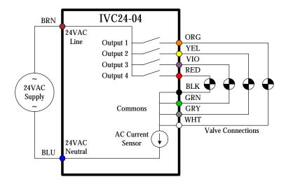
After wiring the device into the system, use a magnet to activate the reed switch "service pin" and send the device's unique ID over the power-line network. Configure the IVC24 from the computer and you are ready to automate your landscape.
